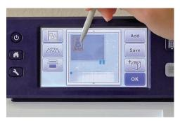
**step 5.** Press the "Embossing" icon (the icon with the "+" sign and box on it) and click on "Line Emboss." Then press the "Settings" icon and change the embossing pressure to "O". Place the desired embossing tool into the embossing tool holder and insert it into the machine.
